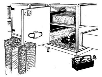
Occasionally, the heat exchanger cells may already be installed in the chamber. They must be taken out before erection of the unit and reinstalled after.
