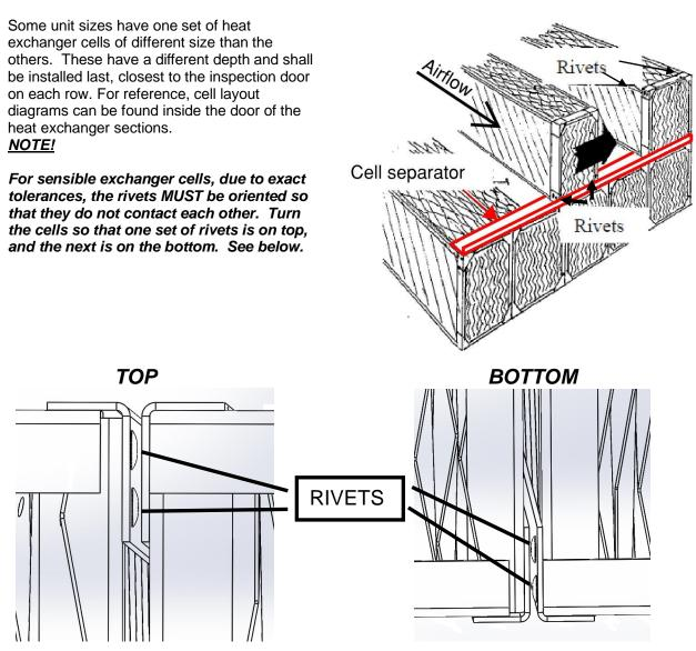
Failure to properly align the rivets can cause the overall width of the heat exchanger cells to increase significantly. The cells will not fit in the drain pan and the door will not close!
