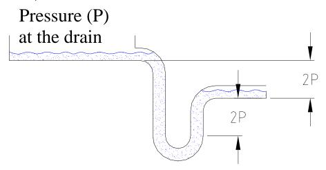
This height will also determine the height H of the mounting framework as detailed on page 6. H should be 4P, plus 2".
