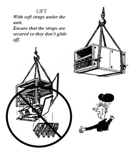
When using lifting lugs to raise the unit, spreader bars must be used to prevent damage to the equipment. If lifting lugs are not present each unit must be lifted with soft straps under the lower framework. Since the profiles used are slippery, the soft straps must be secured to keep the straps from sliding off.
