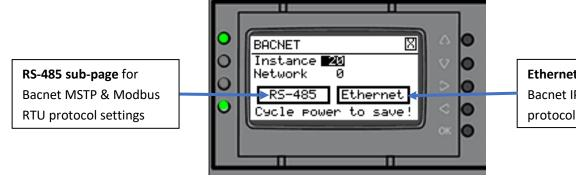
**Ethernet sub-page** for Bacnet IP, FTP, & Http protocol settings
