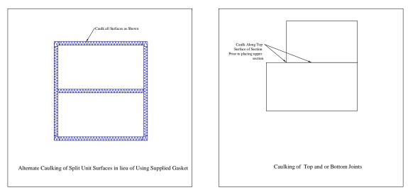
Outdoor units with sections stacked one on top of the other should be caulked prior to placing the section on the other.
